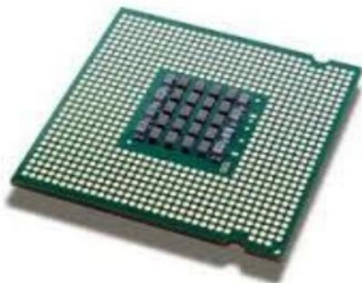
Some microprocessor chips, Fig. 8, can have several million logic gates and a DIL package is not suitable. The active part of the microprocessor “**wafer**” is usually just a **few millimetres** across. However, it can have more than a hundred output pins. Special sockets are often used to wire microprocessors
